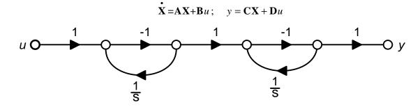
Q.54 The state-variable equations of the system shown in the figure above are
